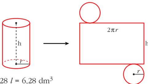
$$\begin{aligned} \text{Área total} &= 2\pi r h + 2\pi r^2 = \\ &= 2\pi r(h + r) \end{aligned}$$
